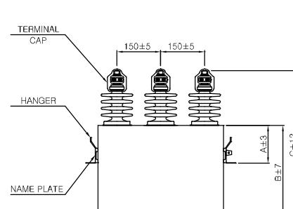
\* Applied bushing could be changed by special requirements [See Table under Bushing Characteristics].
